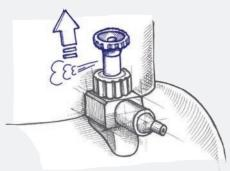
Operating pressure infinitely variable Should the operating pressure in the sprayer exceed the admissible value, the safety valve integrated in each pressure sprayer will automatically correct it. With all pressure sprayers
